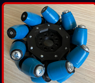
Custom cost-effective mecanum wheels
